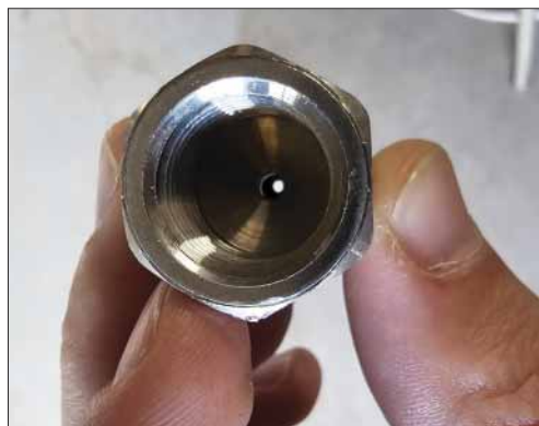
This view of a flow restrictor shows the size of the orifice in a one (1) gpm flow rate.
